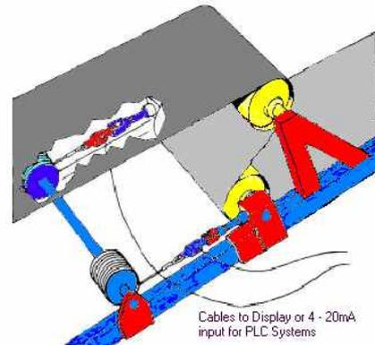
Correct and equal tension will reduce belt wear and tear, reducing ongoing maintenance costs. The Monitoring System pays for itself by protecting the conveyor belt. Models are available to suit the various Conveyor Systems. We have designs for most of these systems. Whilst electric motors have protection via current sensing they cannot operate or monitor the conveyor with the same degree of speed, accuracy or efficiency provided by the installation of Load Cells.
